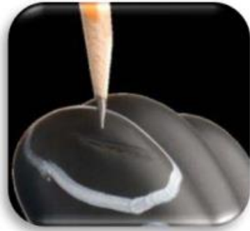
Grooves worn due to rope burns or heat exposure
